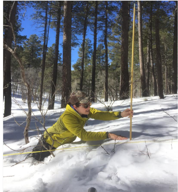
Bethany Coulthard takes a manual snow survey sample on the Mogollon Rim, Arizona in 2016. Image Credit: Joel Biederman.
