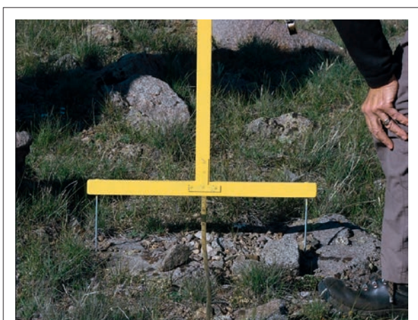
Fig. 7.4 A pointer tool with two sampling pins for sampling a pair of points 0.5m apart.
